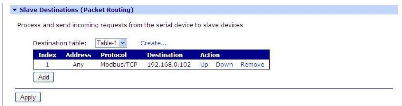
Fig. 25. Example configuration for communication with MODBUS-MASTER devices – table configuration of SLAVE type devices
