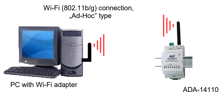
Fig. 4. Connection AD-HOC type between ADA-14110 and PC
