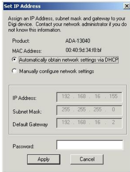
Fig. 13. ADAFinder configuration of IP network address
