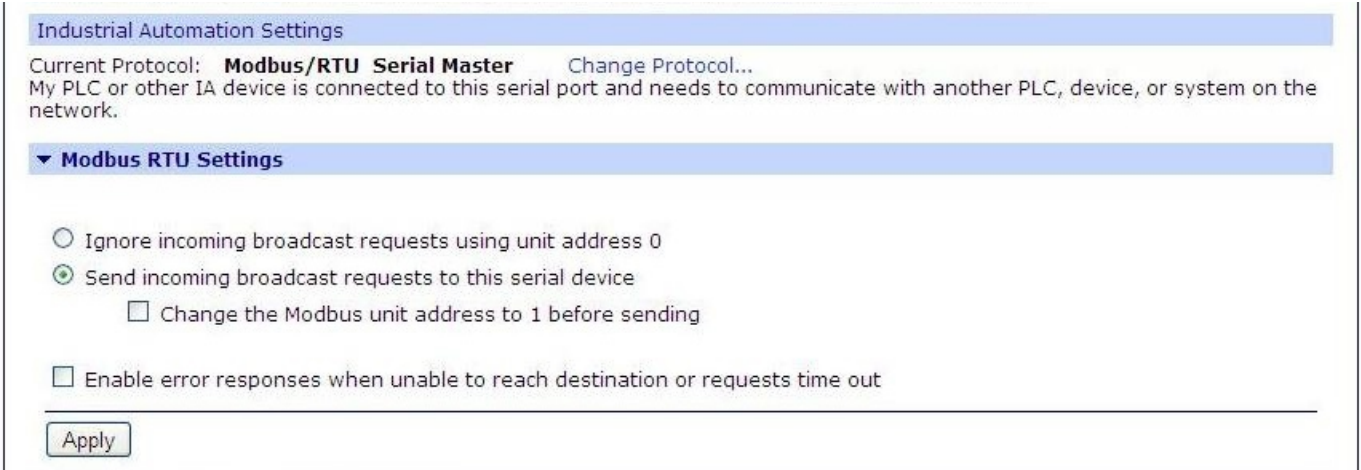
Fig. 22. Example configuration of the converter for communication with a MODBUS-MASTER device – Modbus RTU settings
