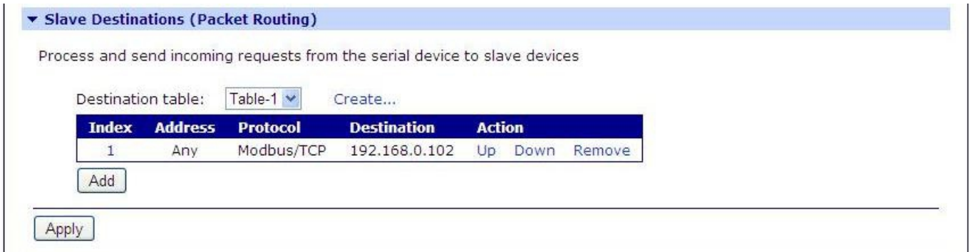
Fig. 23. Example configuration of the converter for communication with a MODBUS-MASTER device – Slave devices table configuration
