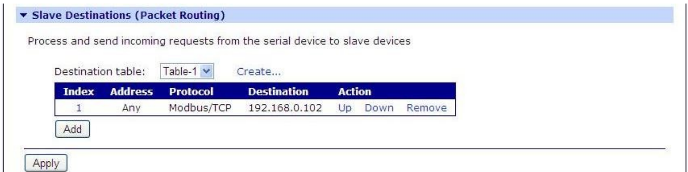
Fig. 27. Example configuration for communication with MODBUS-MASTER devices – table configuration of SLAVE type devices
