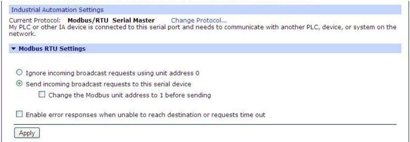
Fig. 26. Example configuration for communication with MODBUS-MASTER devices – Modbus RTU setting
