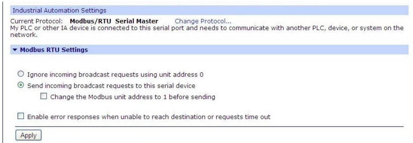
Fig. 24. Example configuration for communication with MODBUS-MASTER devices – Modbus RTU setting
